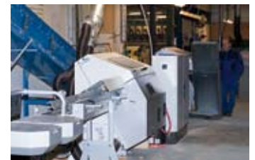
A technician from Paul Saw/Germany fine-tunes the new installation. The optimizing chop saw was custom-built for Wood Castle and installed in December.
