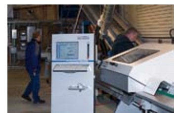
The new saw's sophisticated computer is linked remotely to production managers, facilitating quick and convenient updates to cut lists.
