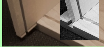
Upper-left: side view of continuous dovetail cut. Main photo: Insertion of drawer panel into sliding dovetail. Inset: Fully inserted panel. Note alignment of drawer bottom dado slots.
