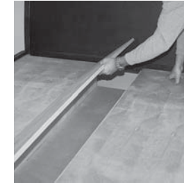
Normally concealed by the mattress, a "secret" storage area nestles between the two side-rail storage units. A removeable middle section of the platform provides the access.
